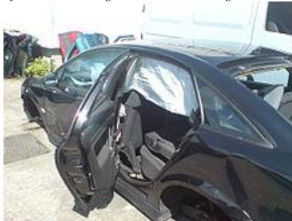
Deployed curtain airbag and side torso airbag in a Citroën C4.
