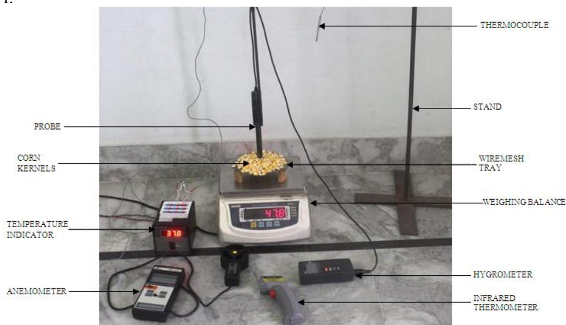
Figure 1: A photograph of experimental set-up for open sun drying mode.
