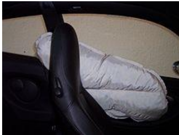
Side airbag inflated permanently for display purposes
