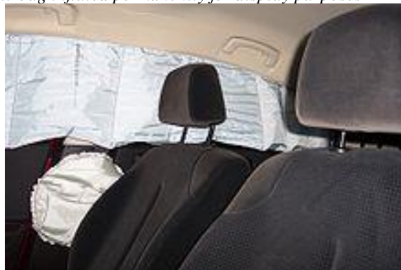
Side airbag inflated permanently for display purposes
