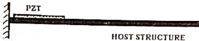
Figure: A typical smart beam with PZT actuator
